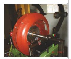
We have various Balancing machines installed at our Works for any type of Rotors weighing upt o 30 Tons as follows:-
